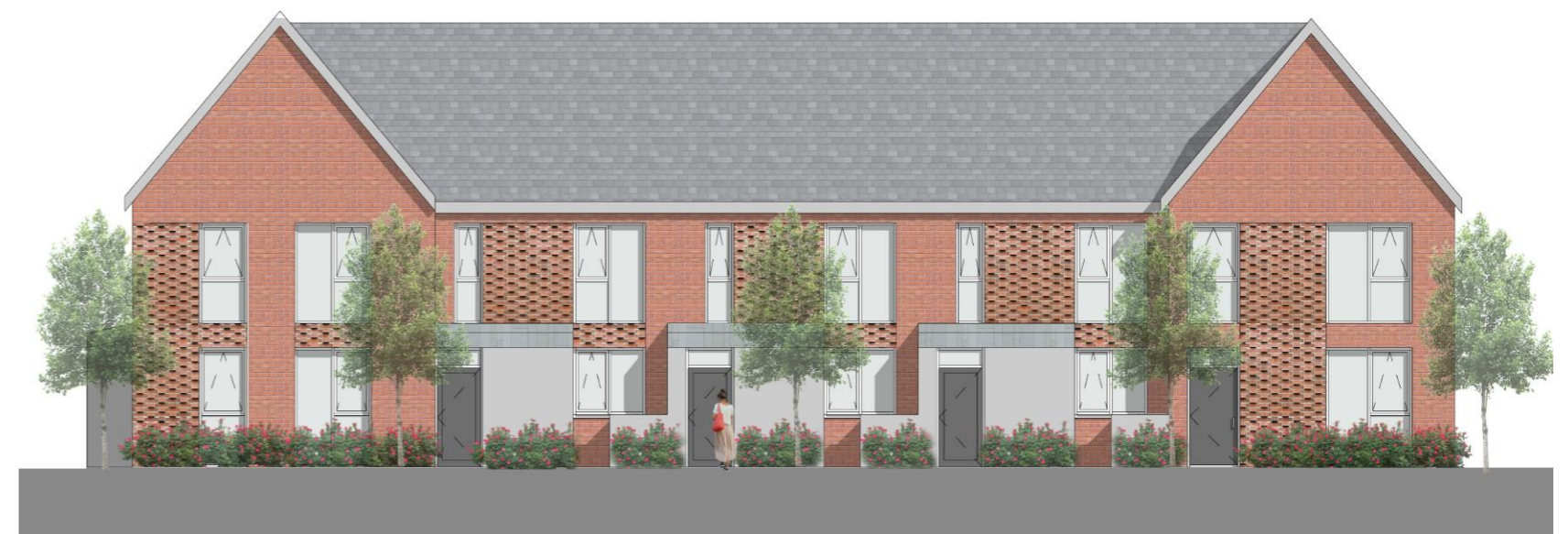
Front Elevation of a typical St. Kevin's townhouse terrace showing warm terracotta brick and protruded brick detail
